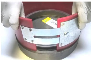
It is always recommended the Duo Cone / Metal Face float Seals must be installed using proper Installation Tool only.
