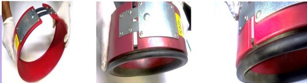
6. Bring the edges of clamp close to each other and tighten the check nut provided on tool so as to hold the seal firmly in the clamp formed.
