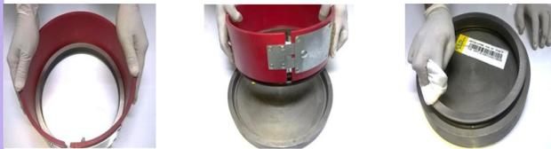
1. For installation of Seal, arrange a cleaned Seal & cleaned ,wiped housing .Put the Seal on the Housing
