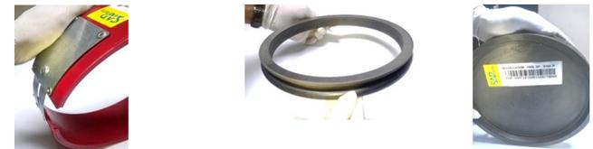
3. Apply Seal-O-Fix on Seal face and clean the Seal using Lint Free Wipe. Ensure the seal face be thoroughly cleaned and no fine particles of dust should remain on it. Employ the spray on the O-Ring circumference, this gives sufficient lubrication for Seal to fit in the cavity of Housing.
