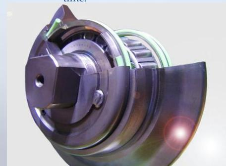
labyrinth created by the hub and seal retainers and then, given time, dries, effectively cementing one metal face seal ring to the other. When the cutter starts rolling again, the cemented metal rings may momentarily spin with each other and stretch the rubber toric holding the metal seal rings. This can rip the toric, allowing leakage of lubricant out of the cutter, as well as ingress of dirt and abrasives into the bearing cavity.
